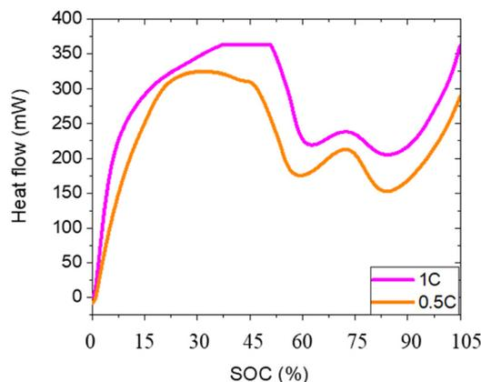
Fig. 3 Comparison of heat generation versus SOC at 0.5C and 1C rates at a temperature of 30 °C.
