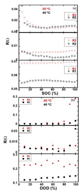
Fig. 4 Individual resistance components at two different temperatures, 20 °C and 40 °C, as a function of (a) SOC and (b) DOD.
