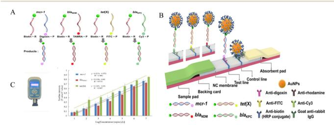
Fig. 7 (A) Scheme of the cascade detection system. Schematic illustration of RPA. (B) HRP-catalyzed LFIA. Reproduced with permission. <sup>64</sup> Copyright 2023, Basel, Switzerland. (C) Quantitative analysis of RPA-LFD. The standard linear equation and correlation coefficient ( $R^2$ ) between the T/C value and the logarithm of the copy number of target DNA (copies per  $\mu$ L). Reproduced with permission.<sup>63</sup> Copyright 2022, Frontiers.
