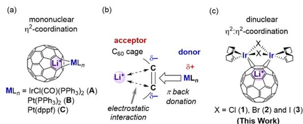
**Fig. 1** (a) Previously-reported  $\text{Li}^+\text{@C}_{60}$ –TM complexes.<sup>9</sup> (b) Schematic diagram of the electrostatic interaction between the  $\text{C}_{60}$  cage and metal fragments  $\text{ML}_n$ . (c) Illustration of the  $\text{Li}^+\text{@C}_{60}$ – $[\text{Ir}_2]$  complexes in this work.
