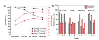
Fig. 2 Catalysis data including: (a) conversion (black) and selectivity (red) of  $NH_2$ -Cr-BDC and amine composites in 1 bar (solid square) and 5 bar (solid circle)  $CO_2$  and (b) the cycling data of the materials in 5 bar  $CO_2$  for 6 b.
