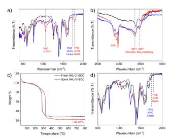
Fig. 3 FTIR data of fresh (black) and spent NH2-Cr-BDC before (red) and after washing (blue) in the range of (a)  $500-2000~{\rm cm}^{-1}$  and (b) 2500-4000 cm $^{-1}$ ; (c) TGA data of fresh (black) and spent NH<sub>2</sub>-Cr-BDC after washing (red) and (d) FTIR data of [amineH+Br-]-Ac-NH-Cr-BDC composities including: fresh TAEA (black), spent ED (red), spent DETA (blue) and spent TAEA (green) samples after 3 cycles of catalysis.
