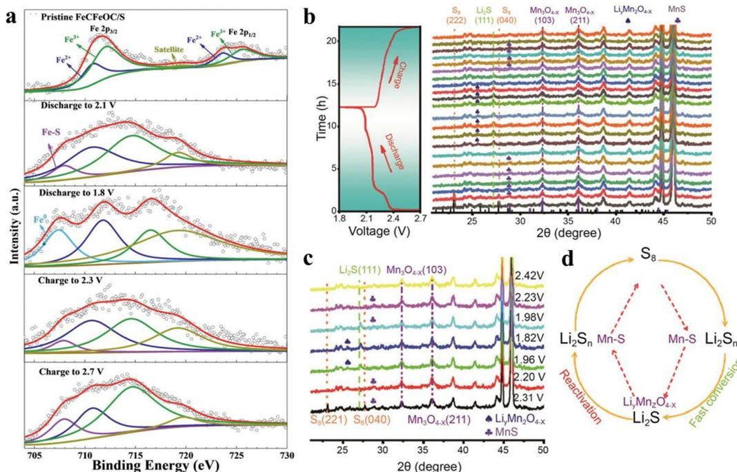
Fig. 3 (a) The Fe 2p XPS spectra of the FeCFEOC/S cathodes. Reproduced with permission from ref. 62 Copyright (2021) Wiley-VCH. (b) *In situ* XRD patterns and the corresponding galvanostatic charge-discharge (GCD) profiles of Mn<sub>3</sub>O<sub>4-x</sub>. (c) Magnified *in situ* XRD patterns. (d) Cycle of sulfur conversion with the Mn<sub>3</sub>O<sub>4-x</sub> catalyst. Reproduced with permission from ref. 50 Copyright (2023) Wiley.
