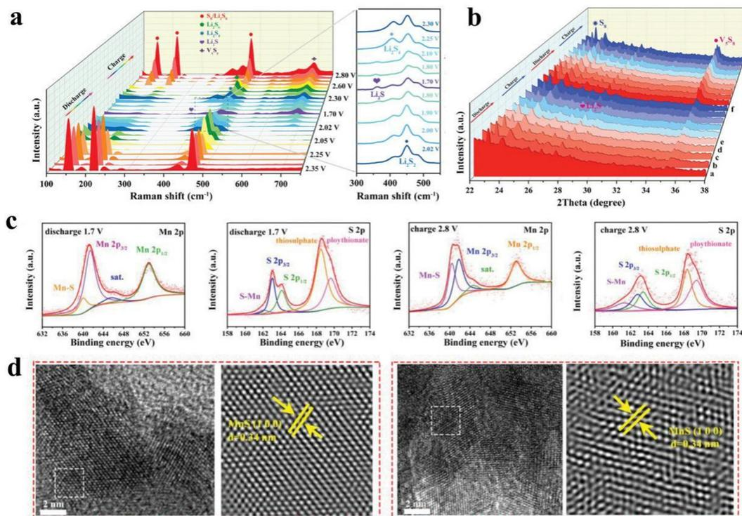
Fig. 4 (a) *In situ* Raman spectra. (b) *In situ* XRD patterns of the VC-VO/HPC@S cathodes. Reproduced with permission from ref. 52 Copyright (2023) Wiley-VCH. (c) Mn 2p, S 2p XPS spectra after discharging to 1.7 V/2.8 V. (d) HRTEM images of MnP-Mn<sub>2</sub>P/C@S cathodes after charging to 2.8 V. Reproduced with permission from ref. 51 Copyright (2023) Wiley-VCH.
