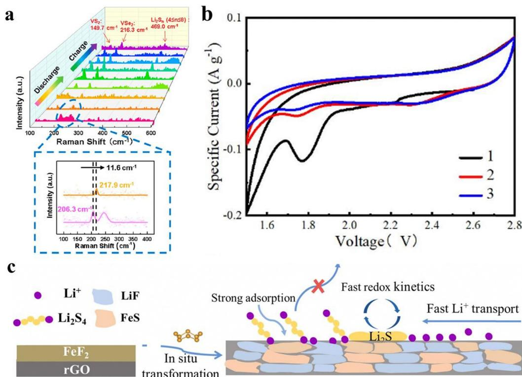
Fig. 5 (a) Operando Raman spectra at different discharge and charge states and the magnified view of the signal of  $\text{VSe}_2$ . Reproduced with permission from ref. 65 Copyright (2020) American Chemical Society. (b) Cyclic voltammetry curve of  $\text{FeF}_2@r\text{GO}$  cathode without sulfur. (c) Schematic diagram of the cathode catalytic conversion process during the cycle. Reproduced with permission from ref. 66 Copyright (2022) Elsevier.
