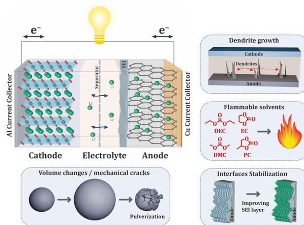
**Fig. 1** Schematic illustration of Li-ion battery working principle. Highlighted dendrite growth, flammable solvents used in electrolytes, volumetric changes leading to the pulverization and interface stabilization.
