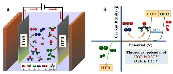
Fig. 1 (a) Schematic of urea-assisted water splitting (urea electrolysis) for hydrogen production. (b) Comparison of polarization curves for UOR, OER and HER.
