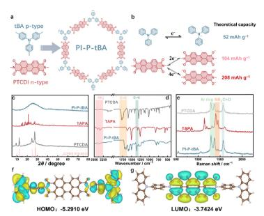
Fig. 1 (a) Structures of tBA, PTCDI and PI-P-tBA, (b) theoretical capacities of tBA and PTCDI in PI-P-tBA (calculation details in Fig. S2, ESI†), (c) XRD patterns, (d) FT-IR and (e) Raman spectra of TAPA, PTCDA and PI-P-tBA, and (f) HOMO and (g) LUMO of PTCDI with two tBA units.
