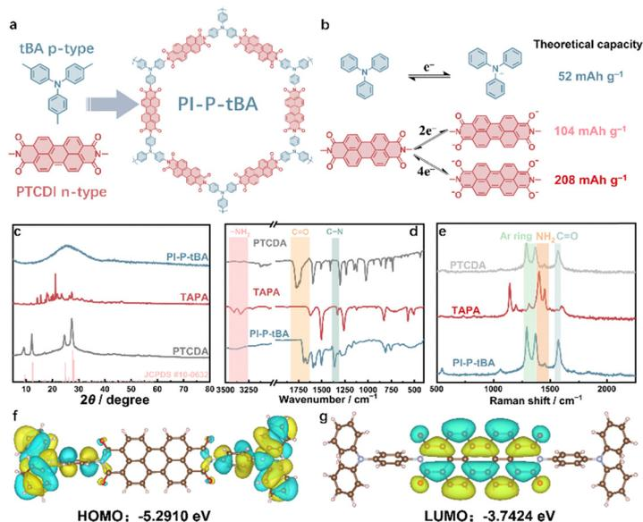
Fig. 1 (a) Structures of tBA, PTCDI and **PI-P-tBA**, (b) theoretical capacities of tBA and PTCDI in **PI-P-tBA** (calculation details in Fig. S2, ESI<sup>†</sup>), (c) XRD patterns, (d) FT-IR and (e) Raman spectra of TAPA, PTCDA and **PI-P-tBA**, and (f) HOMO and (g) LUMO of PTCDI with two tBA units.
