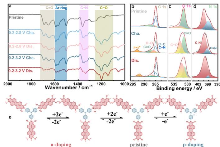
Fig. 3 (a) FT-IR spectra of **PI-P-tBA** in the pristine and charge/discharge states with the voltage ranges of 0.2–2.8 V and 0.2–3.2 V. (b) C 1s, (c) O 1s and (d) N 1s XPS spectra of **PI-P-tBA** in the pristine and charge/discharge states in the voltage range of 0.2–3.2 V. (e) Proposed redox mechanism of **PI-P-tBA**.
