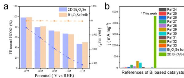
Fig. 2 Effective utilization of the 2D catalyst. (a)  $\text{CO}_2\text{RR}$  to  $\text{HCOO}^-$  performance of 2D  $\text{Bi}_2\text{O}_2\text{Se}$  and  $\text{Bi}_2\text{O}_2\text{Se}$  bulk at 1.01 bar. (b) The comparison of some typical Bi-based 2D catalysts for  $\text{CO}_2\text{RR}$  to  $\text{HCOO}^-$  with 2D  $\text{Bi}_2\text{O}_2\text{Se}$ .
