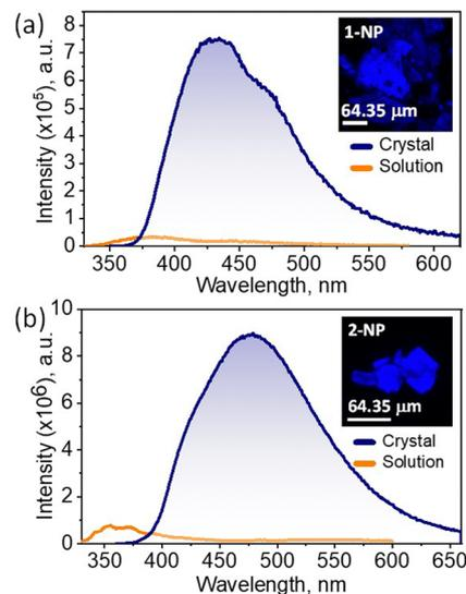
Fig. 2 Fluorescence spectra of (a) **1-NP** and (b) **2-NP** in tetrahydrofuran solution ( $10 \mu\text{M}$ , orange line) and crystalline state (blue line). Inset showing the confocal images of the respective crystals.
