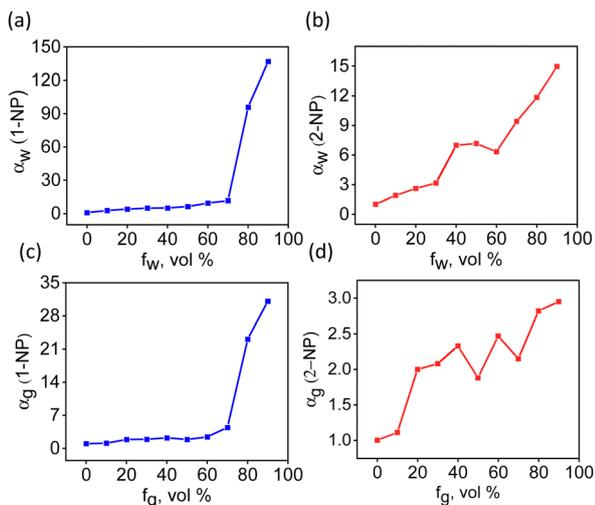
Fig. 3 Relative fluorescence intensity  $\alpha_w$  of (a) **1-NP** and (b) **2-NP** in THF:water mixtures at different water fractions,  $f_w$  ( $\alpha_w = I/I_0$ ,  $I_0$ : Intensity at  $f_w = 0\%$ ). Relative fluorescence intensity  $\alpha_g$  of (c) **1-NP** and (d) **2-NP** in methanol: glycerol mixtures at different glycerol fractions,  $f_g$  ( $\alpha_g = I/I_0$ ,  $I_0$ : Intensity at  $f_g = 0\%$ ).
