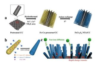
Fig. 6 (a) and (b) Schematic illustrations of the synthesis of the FeCo<sub>2</sub>S<sub>4</sub> nanotube arrays supported on CC through a two-step method by anion exchange reactions. (c) Schematic diagram of the rapid electron/ion transportation within the FeCo<sub>2</sub>S<sub>4</sub> NTA/CC electrode during OER process. Reproduced with permission from ref. 63. Copyright 2019 American Chemical Society.
