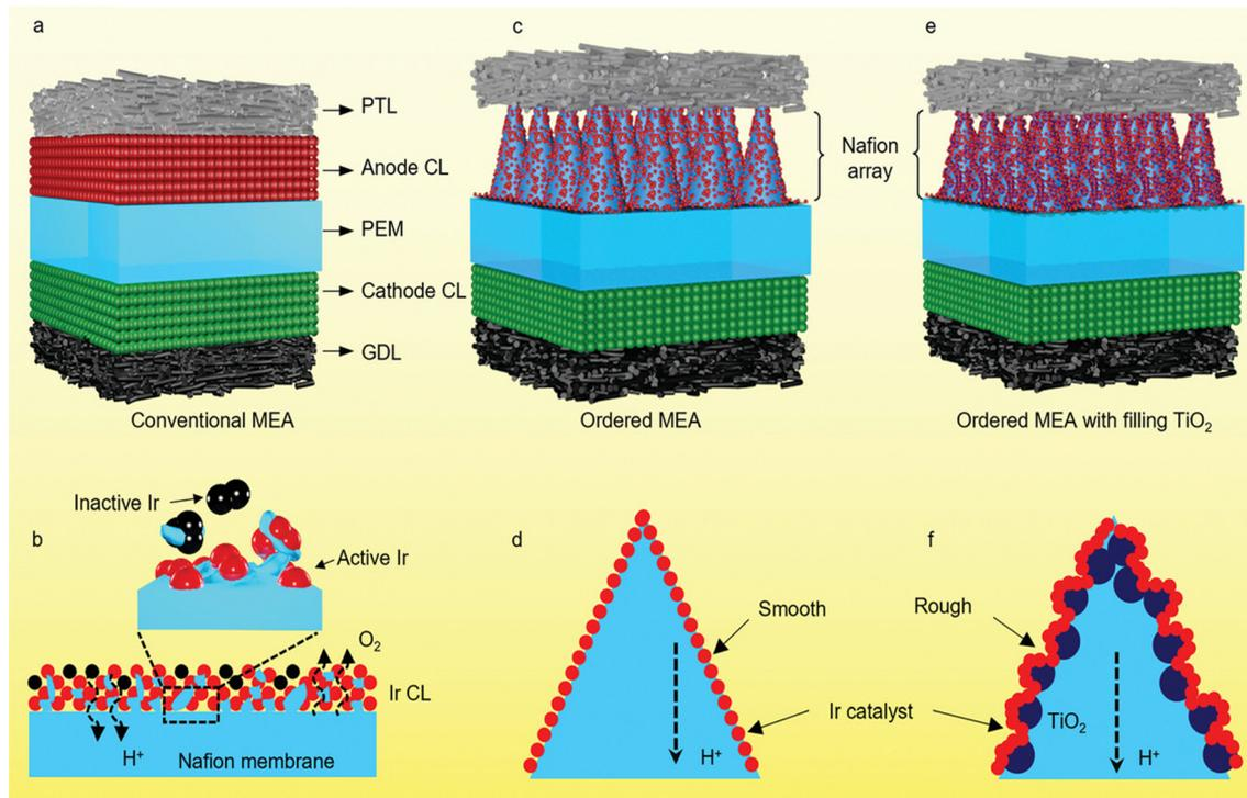
Fig. 14 (a) Conventional MEA. (b) Cross-section images of conventional MEA. (c) Ordered MEA. (d) Cross-section images of ordered MEA. (e) Ordered MEA with  $\text{TiO}_2$  doping. (f) Cross-section images of ordered MEA with  $\text{TiO}_2$  doping. Reproduced with permission from ref. 144. Copyright 2023 Wiley.
