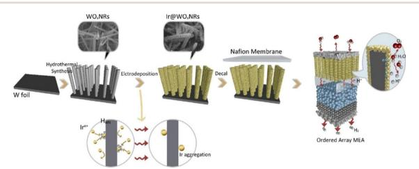
Fig. 8 Schematic diagram of the preparation and structure of the Ir@WOxNR ordered electrode. Reproduced with permission from ref. 82. Copyright 2021 American Chemical Society
