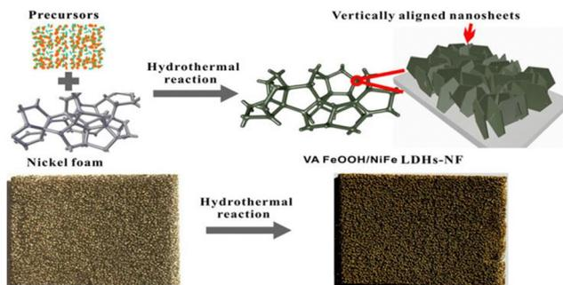
Fig. 9 Schematic illustration of the formation process of the porous VA FeOOH/NiFe LDHs-NF electrodes. Reproduced with permission from ref. 86. Copyright 2016 American Chemical Society.
