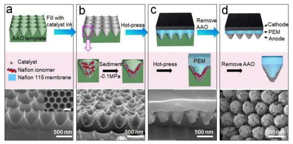
Fig. 13 Preparation procedure of the MEA with GTAs. (a) SEM image of a cross section of the AAO template. The inset shows the top view of the template. (b) Cross-sectional SEM image of the dried template filled with catalyst and ionomer. (c) SEM image of the composite structure of the CL, PEM, and the template. (d) SEM image of the tapered arrays after removing the template. Reproduced with permission from ref. 138. Copyright 2022 American Chemical Society.
