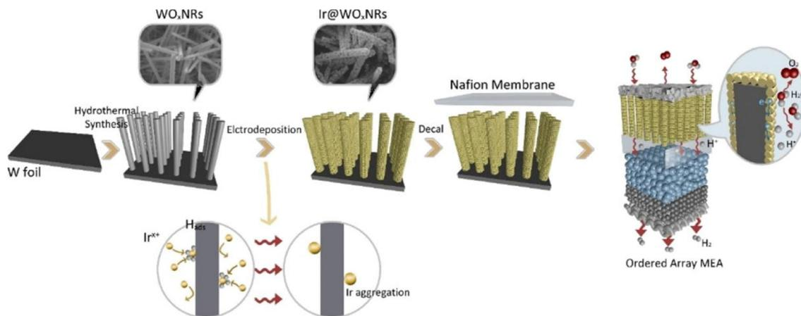
Fig. 8 Schematic diagram of the preparation and structure of the Ir@ $\text{WO}_x\text{NR}$  ordered electrode. Reproduced with permission from ref. 82. Copyright 2021 American Chemical Society.
