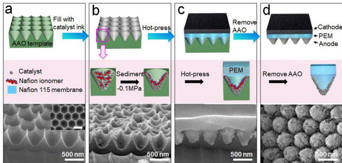
**Fig. 13** Preparation procedure of the MEA with GTAs. (a) SEM image of a cross section of the AAO template. The inset shows the top view of the template. (b) Cross-sectional SEM image of the dried template filled with catalyst and ionomer. (c) SEM image of the composite structure of the CL, PEM, and the template. (d) SEM image of the tapered arrays after removing the template. Reproduced with permission from ref. 138. Copyright 2022 American Chemical Society.
