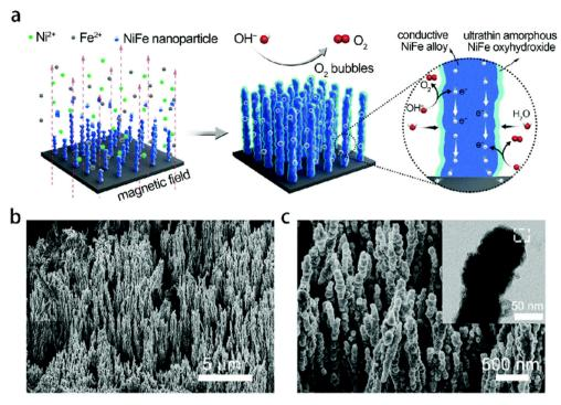
Fig. 5 (a) Schematic of the synthesis of the  $Ni_xFe_{1-x}$ -AHNA nanowire array and its function for OER. (b) and (c) SEM images of  $Ni_xFe_{1-x}$ -AHNAs at different magnifications. The inset of (c) is a low magnification TEM image of a single nanowire. Reproduced with permission from ref. 53. Copyright 2020 Royal Society of Chemistry.
