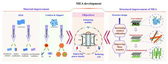
Fig. 4 The trend of the development of nanostructured MEAs. Reproduced with permission from ref. 42. Copyright 2019 Royal Society of Chemistry.
