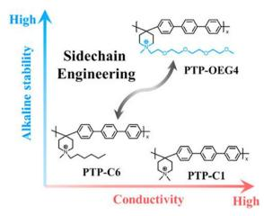
Fig. 12 The impact of side chain engineering on hydroxide conductivity and alkaline stability of AEMs. Reproduced with permission from ref. 130. Copyright 2023 Elsevier.
