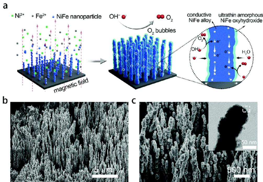
Fig. 5 (a) Schematic of the synthesis of the Ni<sub>x</sub>Fe<sub>1-x</sub>-AHNA nanowire array and its function for OER. (b) and (c) SEM images of Ni<sub>x</sub>Fe<sub>1-x</sub>-AHNAs at different magnifications. The inset of (c) is a low magnification TEM image of a single nanowire. Reproduced with permission from ref. 53. Copyright 2020 Royal Society of Chemistry.
