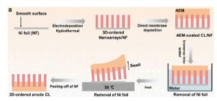
Fig. 11 Schematic diagram for the novel swell-assisted transfer method. Reproduced with permission from ref. 104. Copyright 2024 Royal Society of Chemistry.
