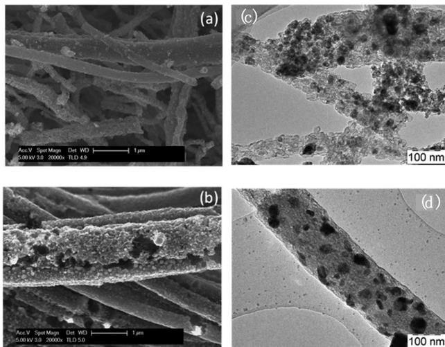
Fig. 7 SEM micrographs of the (a)  $\text{NiCo}_2\text{O}_4/\text{CNF}$  and (b)  $\text{NiMn}_2\text{O}_4/\text{CNF}$  anode catalysts. TEM micrographs of the (c)  $\text{NiCo}_2\text{O}_4/\text{CNF}$  and (d)  $\text{NiMn}_2\text{O}_4/\text{CNF}$  anode catalysts. Reproduced with permission from ref. 72. Copyright 2019 Elsevier.
