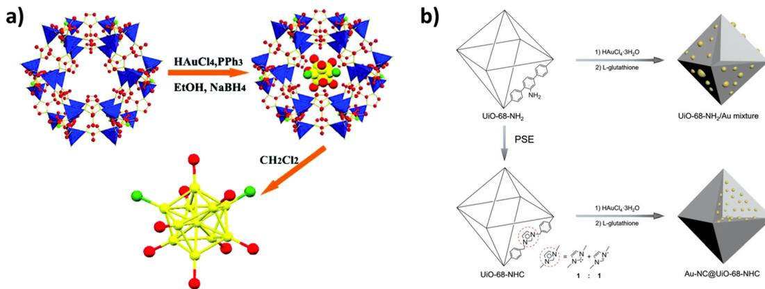
Fig. 4 (a) Schematic representation of the process of Au NCs synthesis in MOFs and the example of  $\text{Au}_{11}@\text{ZIF-8}$ . Reproduced with permission from ref. 66. (b) Schematic illustration of the synthesis of UiO-68-NHC, Au-NC@UiO-68-NHC, and UiO-68-NH<sub>2</sub>/Au mixture. Reproduced with permission from ref. 67.
