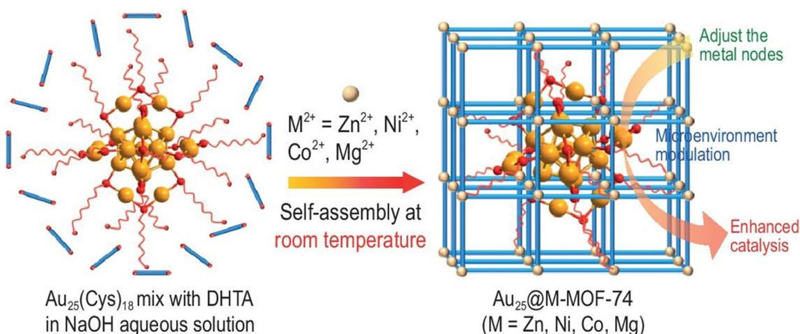
Fig. 6 Schematic illustration showing the synthetic route to Au<sub>25</sub>@M-MOF-74 (M = Zn, Ni, Co, Mg) for enhanced catalysis through microenvironment modulation around Au<sub>25</sub>(Cys)<sub>18</sub> by adjusting the metal nodes on MOF pore walls. Reproduced with permission from ref. 76.
