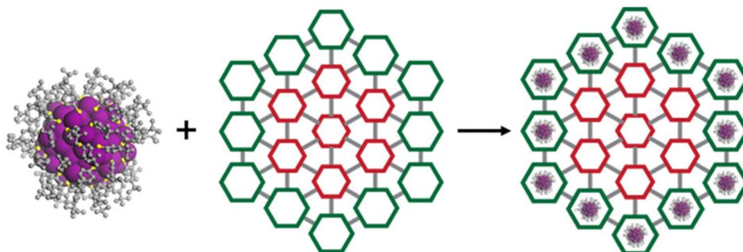
Fig. 3 Schematic representation of “ideal” Au<sub>133</sub>(SR)<sub>52</sub> organization in the periphery of gradient bMOF-102/106. Reproduced with permission from ref. 64.
