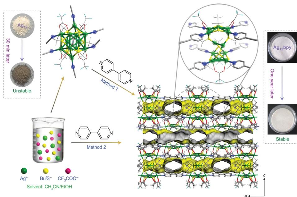
Fig. 7 Schematic illustration of the ligand-exchange strategy (method 1) used to obtain  $\text{Ag}_{12}\text{bpy}$  crystals and one-pot synthesis (method 2) under identical conditions. Reproduced with permission from ref. 77.
