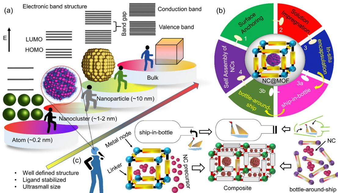
**Scheme 1** (a) Schematic illustration of the size of nanoparticles and nanocluster and representation of electronic structure. (b) Flow chart presenting the strategy adopted for the synthesis of NC and MOF composite functional materials. (c) Schematic presentation of *in situ* encapsulation (ship-in-bottle and bottle-around-ship) methods.
