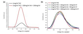
Fig. 4 Comparison of the selectivity of (a) unmodified Metrohm C11L screen printed electrode (b) 2% (w/v) of HMT-PMBI coated on Metrohm C11L screen printed electrode in the presence of ascorbic acid (AA) and caffeine (CF) as interferences (1  $\mu g$  mL $^{-1}$   $\Delta^9$ -THC, TRIS buffer pH 10).
