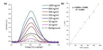
Fig. 3  $\Delta^9$ -THC signals from triplicate experiments performed using 2% (w/v) of HMT-PMBI coated on Metrohm C11L screen printed electrodes in TRIS buffered solution at pH 10 (a) and the linear fit of the  $\Delta^9$ -THC data presenting the corresponding error bars (b), each concentration was performed in triplicate.
