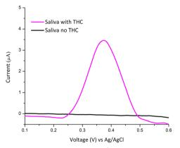
Fig. 5 Differential pulse voltammetry of  $\Delta^9$ -THC in spiked saliva using 2% (w/v) of HMT-PMBI coated on Metrohm C11L screen printed electrode. 1 mL of saliva was spiked with 5  $\mu g$  mL  $^{-1}$  of  $\Delta^9\text{-THC}$  and diluted to a 9 mL solution before testing (550 ng mL<sup>-1</sup>).
