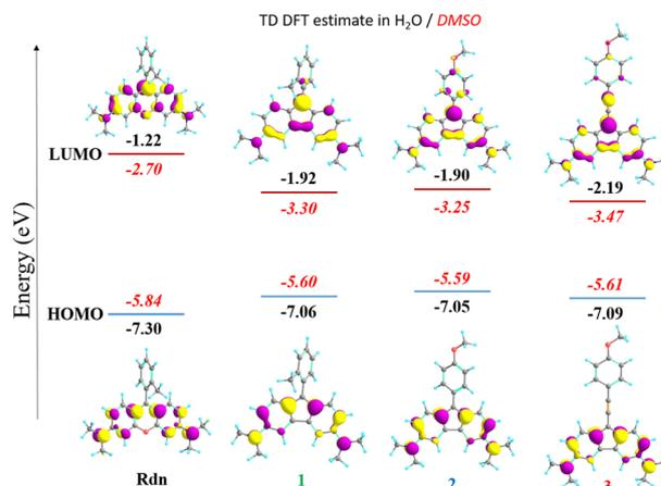
Fig. 3 The frontier molecular orbitals (HOMO/LUMO; isosurface = 0.05 a.u.) with energies (in eV, in H<sub>2</sub>O/DMSO) associated to the  $\lambda_{\text{max}}$  are presented. The effect of the C-9 substituent on the HOMO/LUMO energy levels of the three FluRdn dyes (**1–3**), along with rhodamine (Rdn), is analysed to understand its influence.<sup>38</sup>
