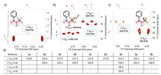
Fig. 3 Excerpts of the HSQC spectra displaying the relevant  $^{1}J_{CH}$  coupling constants for (a) **1a**, (b) **2a**, and (c) **3a** and. (d)  $^{1}J_{CH}$ ,  $^{1}J_{CSI}$  and  $^{2}J_{CSI}$  and  $^{2}J_{CSI}$ values for each alkyl borazines.
