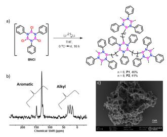
Fig. 5 (a) Synthesis of cross-linked polymers P1 and P2, (b) solid-state  $^{1}\text{H} \rightarrow ^{13}\text{C}$  cross-polarization and magic angle spinning (CPMAS) NMR spectrum of P1, and (c) SEM images of P1 (see CPMAS NMR spectrum for reference borazine 2a in Fig. S68, ESI†).
