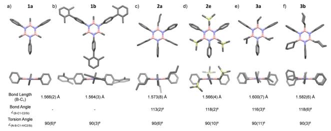
Fig. 2 Single-crystal X-ray structures of borazines and relevant structural parameters (a) 1a, C2/c, (b) 1b, C2/c, (c) 2a, Cc, (d) 2e, P2<sub>1</sub>/c, (e) 3a, P\(\bar{1}\), and (f) 3b, Pna2<sub>1</sub>. Grey: C, pink: B, yellow: Si, and blue: N. The torsion angles are the average of the values measured for C-H/C/Si bonds that display an orientation that is close to that of perpendicularity.
