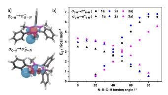
Fig. 4 (a) NBO for  $\sigma_{C-H} \to \pi_{B-N}^*$  and  $\sigma_{C-H} \to \sigma_{B-N}^*$  1a (PBE/def2-TZVP, orbitals with only one B-atom are shown), (b) hyperconjugative energies upon rotation of the B-alkyl group.
