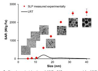
Fig. 5 Size-dependent heating of MNPs. SAR was measured for MNPs ranging from 6 to 40 nm dispersed in DI water, using an AMF at 325 kHz and 20.7 kA m<sup>-1</sup>. The solid curve represents the theoretical SAR predictions according to the LRT model. (Reproduced with permission from ref. 25, ©2017 American Chemical Society)
