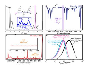
Fig. 3 (A)  $^1\text{H-NMR}$  of PS-co-tBLp after degradation. (B) FT-IR of PS-cotBLp after degradation. (C) Raman spectrum of PS-co-tBLp after degradation. (D) Molecular weight differential distribution curves of PS-co-tBLp-1 before and after ultraviolet photodegradation and DTT catalytic thermal degradation. (PS-co-tBLp-1: [St]<sub>100</sub>/[t-BLP]<sub>2</sub>/[KPS]<sub>2</sub>).
