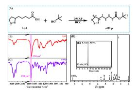
Fig. 1 (A) The synthesis of tert-butyl lipoate. (B) FT-IR of lipoic acid (LpA). (C) FT-IR of tert-butyl lipoate (t-BLp). (D) <sup>1</sup>H-NMR of tert-butyl lipoate. (E) HPLC of tert-butyl lipoate.
