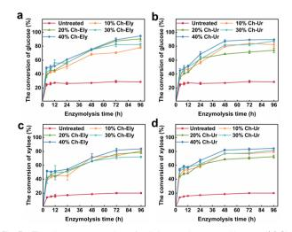
Fig. 3 The glucose conversion of cellulose and untreated bagasse (a) Ch-Ely and (b) Ch-Ur. The xylose conversion of cellulose and untreated bagasse. (c) Ch-Ely and (d) Ch-Ur.
