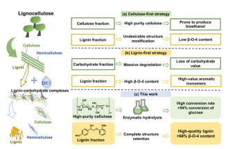
(a) Cellulose-first strategy. (b) Lignin-first strategy. (c) The whole component utilization of biomass strategy proposed in this work using the tailored alkaline DES process.
