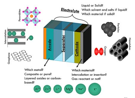
Fig. 12 The basic variables involved in the battery cells (reproduced with permission from Wiley, Copyright © 2022). 215
