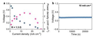
Fig. 4 (a) Polarization and power density curves, and (b) long-term chronopotentiometry curve under 10 mA cm<sup>-2</sup> output of a N<sub>2</sub>H<sub>4</sub>-nitrate batterolyzer.
