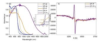
Fig. 2 Absorption spectra of model compounds DT-M, DP-M and polymers DT-P, DP-P & and the iodine doped DT-P (DT-P-I2) (a), Inset: Kubelka Munk plot of DT-P and DP-P. (b) EPR spectra of DT-P in its pristine and doped states.
