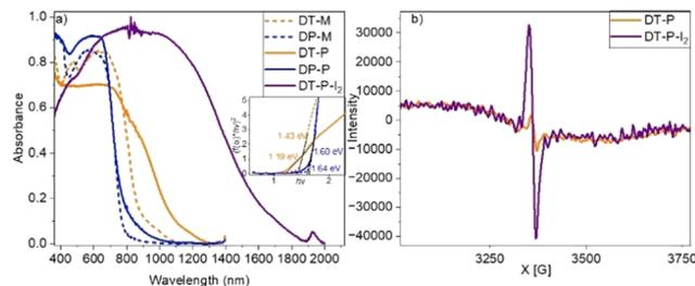
Fig. 2 Absorption spectra of model compounds **DT-M**, **DP-M** and polymers **DT-P**, **DP-P** & the iodine doped **DT-P** (**DT-P-I<sub>2</sub>**) (a), Inset: Kubelka Munk plot of **DT-P** and **DP-P**. (b) EPR spectra of **DT-P** in its pristine and doped states.
