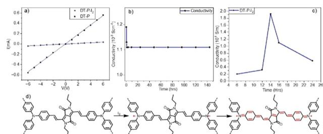
Fig. 3 The *I*–*V* plot of the **DT-P** polymer (a); stability test of the doped **DT-P** polymer (b); conductivity of the **DT-P** polymer at different doping times (c) and the proposed mechanism for the I<sub>2</sub> doped **DT-P** polymer (d).
