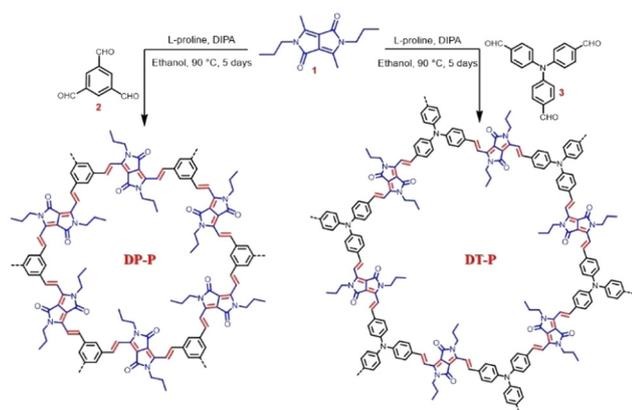
Scheme 1 Synthesis of **DP-P** and **DT-P** CMPs *via* Knoevenagel condensation.
