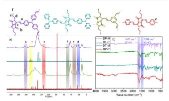
(a) <sup>13</sup>C CPMAS spectra (b) FTIR spectra of **DP-P** and **DT-P** along with their model compounds (DP-M, DT-M).
