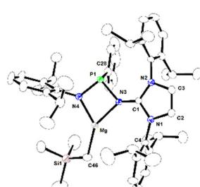
Fig. 2 The molecular structure of Mg-complex **1** with the thermal displacement parameters drawn at 30% probability. Hydrogen atoms are omitted for clarity. Selected bond lengths [Å] and bond angles [°]: Mg–N4 1.9922(16), Mg–N3 2.0832(14), Mg–C46 2.100(9), P1–N4 1.6732(14), P1–N3 1.7607(14), C46–Si1 1.786(9), N3–P1–N4 92.34(7), N3–Mg–N4 74.86(6), N4–Mg–C46 136.2(3), N3–Mg–C46 144.9(4), P1–N4–Mg 99.26(7), P1–N3–Mg 93.14(6), Mg–C46–Si1 116.2(6). CCDC No. 2387519.
