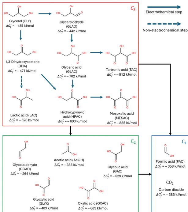
Fig. 1 Reaction pathway for the possible products of electrochemical glycerol oxidation, including the standard Gibbs free energy of formation ( $\Delta_r G^\circ$ ) calculated at 298.15 K and 1 bar at infinite dilution in water.
