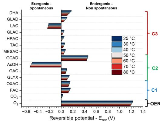
Fig. 2 Reversible potential ( $E_{\text{rev}}$ ) at different temperatures for the oxidation of glycerol to different products (values can be found in Table S5, ESI†).
