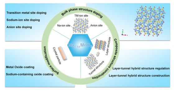
Fig. 6 Summary diagram of the modification strategies for tunnel-structured Na<sub>0.44</sub>MnO<sub>2</sub> cathode material in SIBs.
