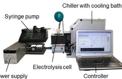
Fig. 8 Automated electrochemical assembly for the synthesis of oligosaccharides.
