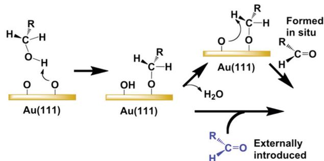
Fig. 2 Schematics of aldehyde formation on O/Au(111) via two pathways: the  $\beta$ -H elimination (top pathway) of alkoxy or introduced externally (bottom pathway, blue). Adapted with permission from ref. 39. Copyright 2010 American Chemical Society.
