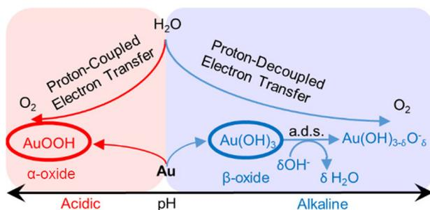
Fig. 4 Proposed mechanism for electrocatalytic water oxidation on gold. In the high-pH region, the rate-limited step of oxygen evolution is deprotonation of Au(OH)<sub>3</sub> involving a decoupled proton-transfer step. Adapted with permission from ref. 57. Copyright 2020 American Chemical Society.
