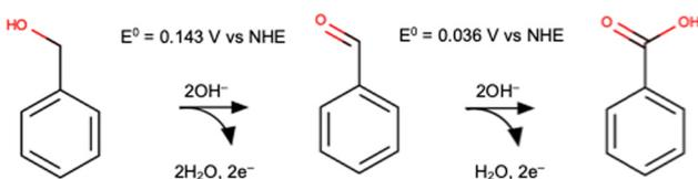
**Scheme 1** Electrochemical oxidation of benzyl alcohol in alkaline electrolytes which generates benzaldehyde and benzoic acid. The standard potential for the oxidation reaction shown corresponds to the anode potential that will lead to an isoergic equilibrium ( $\Delta G^\circ = 0$ ) between the oxidized and reduced molecule under standard state conditions, when protons are reduced to H<sub>2</sub> at the cathode.<sup>27</sup>
