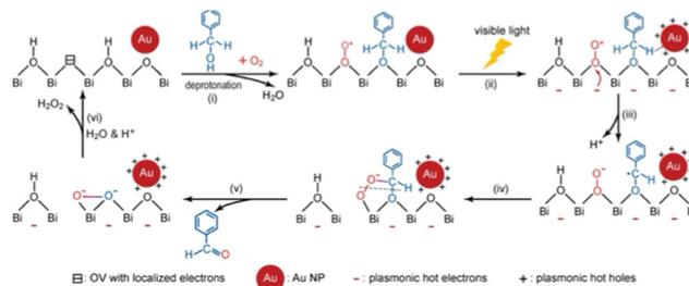
Fig. 11 Proposed reaction mechanism of selective benzyl alcohol oxidation over Au-BiOCl. Adapted with permission from ref. 80. Copyright 2017 American Chemical Society.
