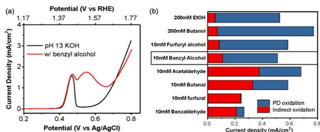
Fig. 6 (a) Cyclic voltammograms of electrochemical oxidation of benzyl alcohol in alkaline electrolytes and (b) the deconvoluted reaction mechanism for 10 mM benzyl alcohol electrochemical oxidation. Adapted with permission from ref. 9. Copyright 2020 American Chemical Society.
