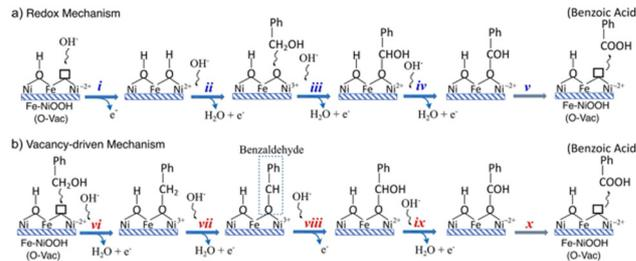
Fig. 7 Benzyl alcohol oxidation mechanisms and their corresponding free energy pathways on the edge site of  $\beta$ -NiOOH (with or without Fe-doped). Schematic representation of reaction intermediates for the benzyl alcohol oxidation process *via* the (a) redox mechanism and (b) vacancy-driven mechanism. Adapted with permission from ref. 7. Copyright 2023 American Chemical Society.
