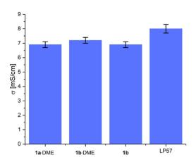
Fig. 2 Bulk conductivities of 1 M Li[B(hfip)<sub>4</sub>]·DME (1a·2DME), 1 M Li[Al(hfip)<sub>4</sub>]·DME (**1b**·DME), 1 M Li[Al(hfip)<sub>4</sub>] (**1b**) and 1 M LiPF<sub>6</sub> (LP57) in EC: EMC (3:7 v/v) solvent, measured at 20 °C. Error bars correspond to error in the EIS fitting
