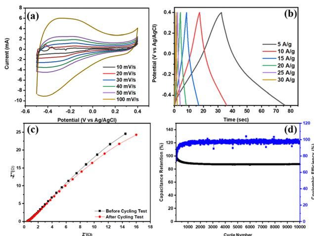
Fig. 3 (a) CV curve at scan rate of 10, 20, 30, 40, 50 and  $100 \text{ mV s}^{-1}$ . (b) GCD profile at current density of 5, 10, 15, 20, 25, and  $30 \text{ A g}^{-1}$ . (c) Nyquist plot before and after cycling stability test. (d) Cyclic stability and coulombic efficiency tested for  $\text{Ti}_3\text{C}_2\text{T}_x$  electrode for 10 000 cycles.
