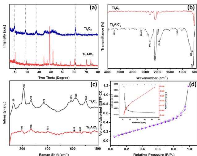
Fig. 1 (a) XRD peak obtained for  $\text{Ti}_3\text{AlC}_2$ -MAX phase and  $\text{Ti}_3\text{C}_2\text{T}_x$  (b) FTIR spectra (c) Raman peak obtained for MAX phase MXene (b) nitrogen adsorption and desorption isotherms of the  $\text{Ti}_3\text{C}_2\text{T}_x$ .
