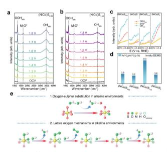
Fig. 1 (a) and (b) In situ FT-IR spectra of (NiCo) $S_{0.89}$  and (NiCo) $S_{1.33}$ . (c) Signal strength variation diagram of characteristic FT-IR peaks of OOH<sub>ads</sub>,  $M\!-\!O^{\star}$  and  $OH_{ads}.$  (d) The ratio of the LOM pathway. (e) Schematic diagram of the LOM mechanism with a lattice sulfur-oxygen substitution process. Reproduced with permission of ref. 45 copyright 2023, Nature Publishing Group.
