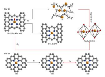
Fig. 2 Coordination or structural changes of the sites S1 and S2 under  $\it operando$  conditions in the electrochemical ORR process.  $^{46}$  Copyright 2021, Springer Nature.
