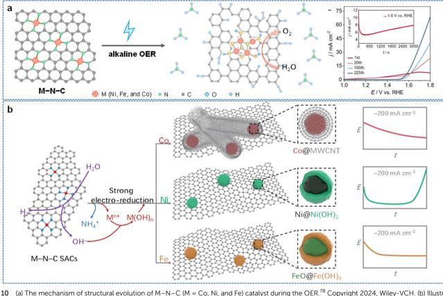
Fig. 10 (a) The mechanism of structural evolution of M-N-C (M=Co, Ni, and Fe) catalyst during the OER. <sup>78</sup> Copyright 2024, Wiley-VCH. (b) Illustration of the mechanism of structural degradation of M-N-C catalysts after long-term and industrial-grade current density HER. 77 Copyright 2024, Wiley-VCH.
