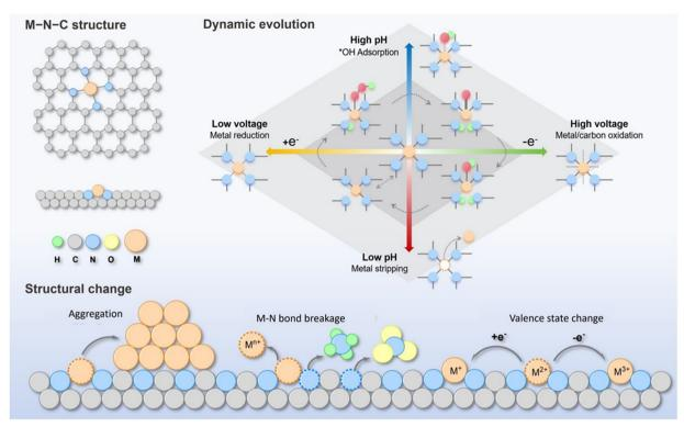
Fig. 8 Schematic illustration of voltage/pH-driven structural evolution of M-N-C catalysts
