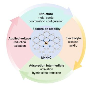
Fig. 1 Factors on the stability of M-N-C catalysts.
