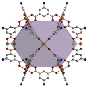
**Fig. 1** Structure of the cuboctahedral  $\text{Mo}_{24}(\text{5-NH}_2\text{-bdc})_{24}$  cage where orange, red, gray, and blue spheres represent molybdenum, oxygen, carbon, and nitrogen, respectively. Hydrogen atoms and metal-coordinated solvent molecules have been omitted for clarity.
