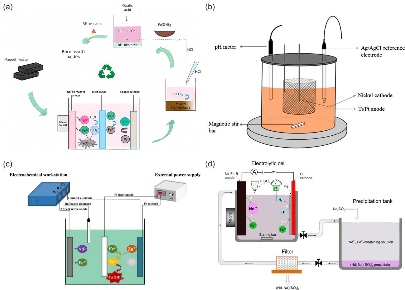
Fig. 9 Schematic representation of (a) recovering RE oxides from NdFeB magnet waste using a dual anode electrolysis reactor, (b) the electrolysis cell for *in situ* electrochemical oxidation of Fe<sup>2+</sup>, (c) a dual anode electrolysis device for recovering REEs from NdFeB magnets (CE, counter electrode; RE, reference electrode; and WE, working electrode) and (d) the closed-loop recycling route for recovering REEs from the NdFeB magnet waste. Reproduced with permission from ref. 51–54.
