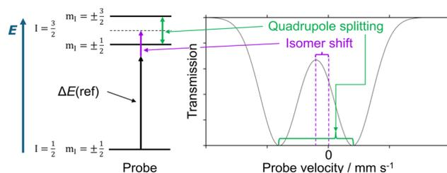
**Fig. 1** Right: Exemplary Mössbauer doublet signal plotted as transmission vs. probe velocity. The isomer shift (violet) refers to the center of the doublet with respect to a reference (typically,  $\alpha$ -iron). The quadrupole splitting (green) measures the separation of the doublet minima. Left: Diagram with the nuclear energy levels; labels refer to the nuclear spin quantum number  $I$  and the nuclear magnetic quantum number  $m_I$ .
