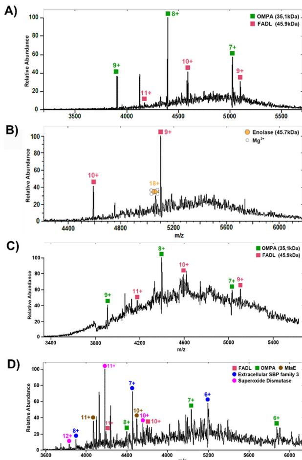
Fig. 1 Representative full-scan mass spectrum obtained following eight rounds of washing (A) and (B) and four rounds (C) and (D) of washing. (A) Mass spectrum with compensation scaling factor 5%. (B) Mass spectrum with CSF 7%. (C) Mass spectrum with CSF 5%. (D) Mass spectrum with CSF 7%.
