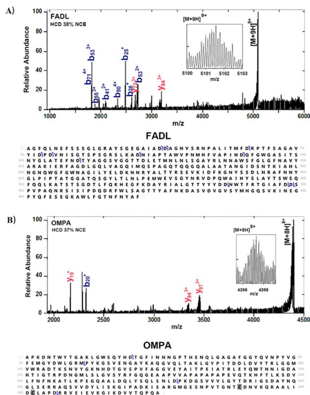
Fig. 2 Identification of FADL and OMPA following the  $2 \times (3 + 1)$  washing protocol. (A) HCD mass spectrum of 9+ ions (see inset) of FADL ( $m/z$  5102  $\pm$  5), NCE38%, and sequence coverage. (B) HCD mass spectrum of 8+ ions (see inset) of OMPA ( $m/z$  4397  $\pm$  5), NCE 37%, and sequence coverage.
