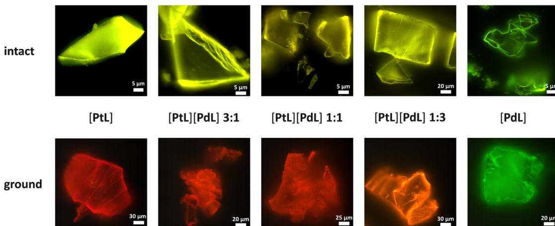
Fig. 2 Micrographs of **[PtL]**,<sup>24</sup> **[PdL]**<sup>24</sup> and their statistical co-crystals with different compositions before (top) and after (bottom) grinding.
