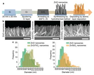
Fig. 2 Metal oxide nanowire fabrication and characterization. (a) ZnO nanowires were synthesized by a hydrothermal method on a silicon substrate having a sputtered chromium (Cr) layer, and the TiO2 and SiO2 layers were deposited on ZnO nanowires by ALD. (b) FESEM images and (c) the histograms of nanowire diameter comparing ZnO nanowires before and after depositing TiO2 or SiO2 layers. Lines indicate the fitting Gaussian distribution (n = 100 nanowires).
