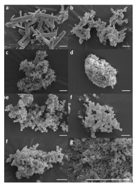
Fig. 2 Scanning electron microscopy images of MIL-68(In) A-D and ZIF-8 E-H with increasing degrees of modulation down the figure. All scale bars represent 5 um.
