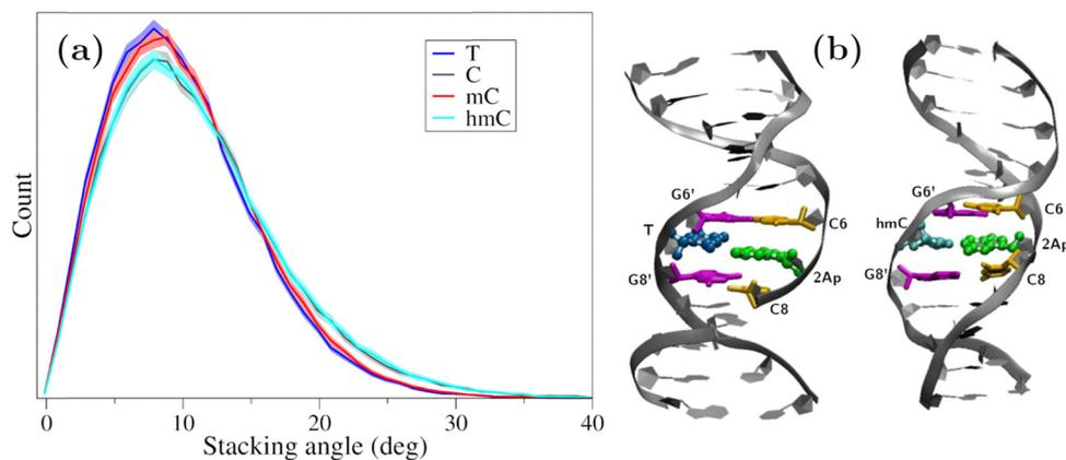
Fig. 3 (a) Stacking-angle distributions between 2Ap and C8 for duplexes containing the different X bases. Average angles are  $10.0^\circ$  (T),  $11.0^\circ$  (C),  $10.2^\circ$  (mC), and  $11.1^\circ$  (hmC). Shaded regions denote 95% confidence intervals obtained from block-bootstrap analysis. (b) Representative structures for T and hmC, including the labels for the nearby bases (color code: C6/C8 in orange, 2Ap in green; G6/G8 in magenta; T in blue, and hmC in cyan).
