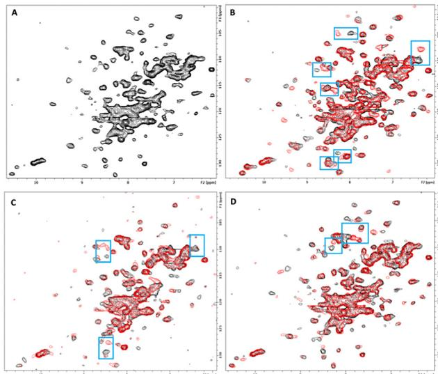
Fig. 4 NMR spectral analysis of the CBL-c TKB domain. (A) The  $^1\text{H}$ - $^{15}\text{N}$  SOFAST HMQC spectrum of the TKB domain of CBL-c. (B) Shifts in CBL-c are induced by interaction with an EGFR peptide fragment EDSFLQR-pYSSDPT. Shifts induced by a fragment mixture (C) and fragment **1** (D) binding to CBL-c.
