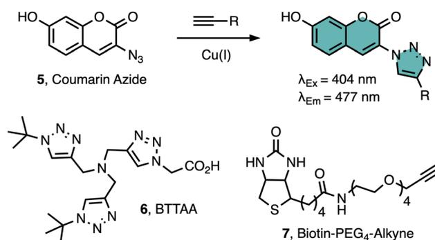
**Scheme 1** Schematic of the fluorogenic assay to monitor product formation under different CuAAC conditions. Also shown are the structures of the Cu<sup>I</sup>-stabilizing ligand BTAA (6) and biotin-PEG<sub>4</sub>-alkyne (7).
