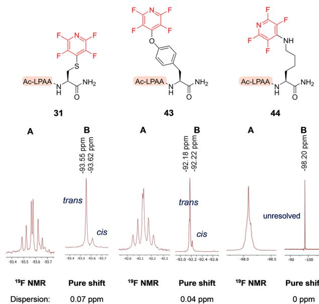
Fig. 4 <sup>19</sup>F NMR spectra of Ac-LPAAX-NH<sub>2</sub> peptide models tagged with **16** (not to scale). (A) with F–F coupling and (B) after pure shift F–F decoupling.
