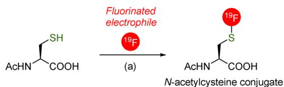
Scheme 2 Reaction screening of fluorine tags. Reagents and conditions: (a) fluorine tag (2 eq.), N-acetyl cysteine (1 eq.), DIPEA (5 eq.), water–acetonitrile (1 : 1), 23 °C, 4 h.
