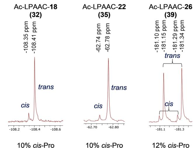
Fig. 3 Example <sup>19</sup>F NMR spectra of tagged Ac-LPAAC (not to scale).
