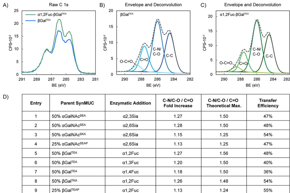
Fig. 3 Application of XPS to quantify the extent of enzymatic synMUC fucosylation or sialylation *via* changes in bond species ratios. Representative XPS raw C 1s spectra of (A) 50%  $\beta$ Gal<sup>TEA</sup> before and after  $\alpha$ 1,2 fucosylation, (B) and (C) deconvolution of C 1s curves into their constituent C–C, C–N/C–O, and C=O peaks plotted under their calculated C 1s envelope curve. (D) Summary of XPS results for enzymatically sialylated and fucosylated synMUCs.
