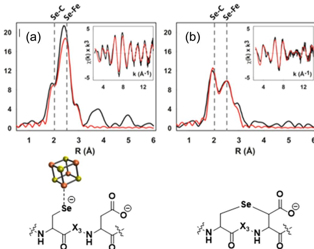
Fig. 12 Se edge EXAFS of PapB reacted with a SeCys-substituted substrate peptide. (a) An intense Se–Fe peak is observed at 2.4 Å when peptide is added in the absence of SAM and DTT. (b) Reaction in the presence of SAM and DTT shows an increase in the Se–C and decrease in the Se–Fe as peptide is converted into the crosslinked product.
