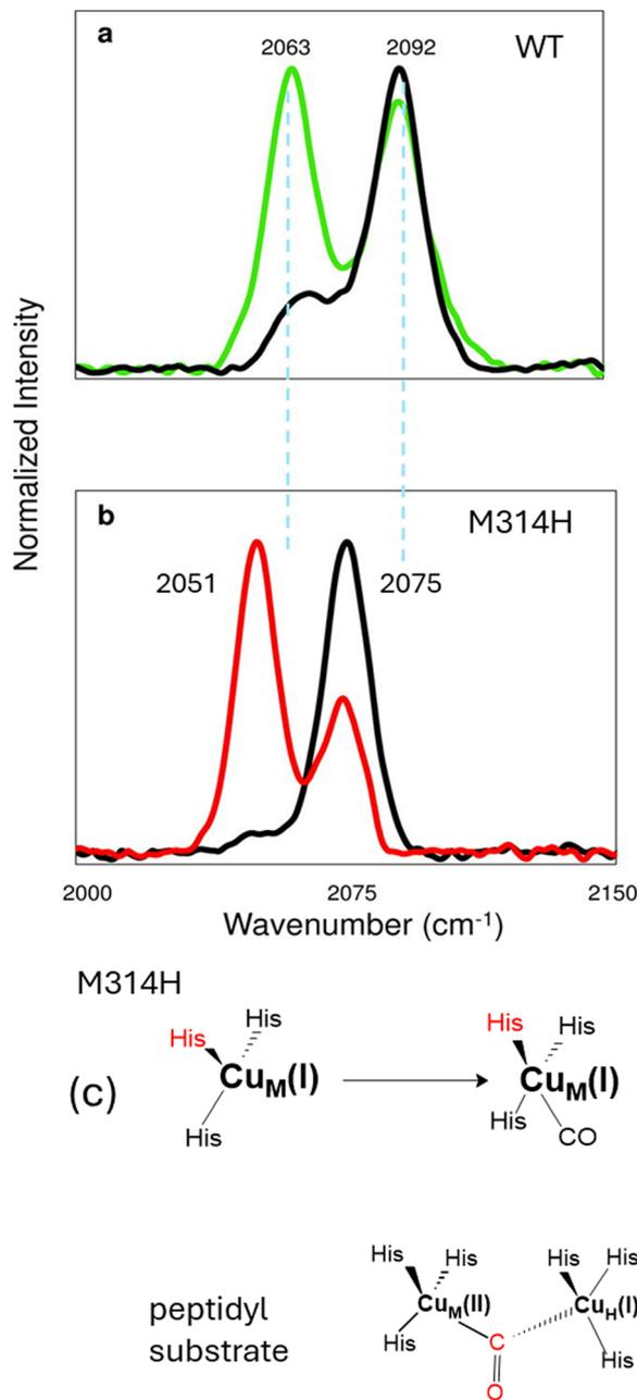
Fig. 4 CO chemistry of Cu(I)-PHM. (a) FTIR of substrate-free (2092  $\text{cm}^{-1}$ ) and substrate-bound (2063  $\text{cm}^{-1}$ ) enzyme. (b) CO complexes of the M314H variant showing both frequencies red-shifted by the Met to His substitution. (c) Suggested semi-bridged arrangement for the substrate-bound complexes.
