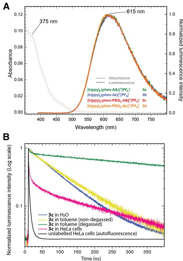
Fig. 3 (A) Absorbance (dashed line) and normalized luminescence upon excitation at 375 nm (solid line) of probes **3a–d** in water. (B) Emission decay at 375 nm excitation for **3c** in water and toluene (non-degassed and degassed by bubbling argon), and in cells, versus emission decay of cell autofluorescence. Note: The decay in cells presents a fast component due to cell autofluorescence and a long component due to the Ir(III) probe.
