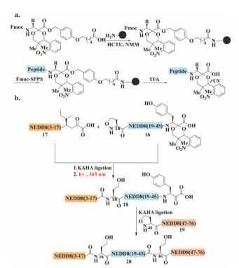
Fig. 8 General schematic presentation for (a) the preparation of the photo-protected  $\alpha$ -ketoacid and (b) NEDD8 synthesis through N- to C-NCL reaction, using three segments and two ligations where photo-protected  $\alpha$ -ketoacid was introduced to peptide **16**.
