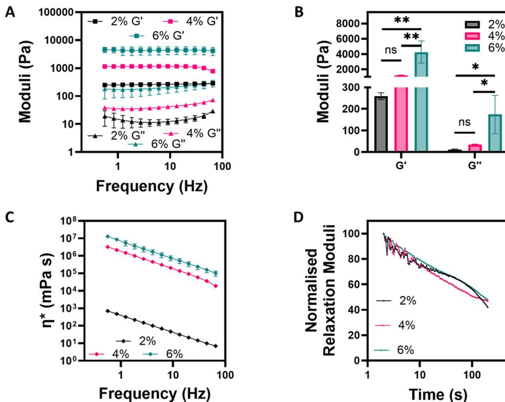
**Fig. 2** Rheological characterisation of methacrylate alginate. (A) Frequency sweeps, (B) storage ( $G'$ ) and loss ( $G''$ ) moduli, (C) complex viscosity, and (D) normalised stress relaxation of ALMA hydrogels. Frequency sweeps and stress relaxation were performed within LVE region (5% strain).
