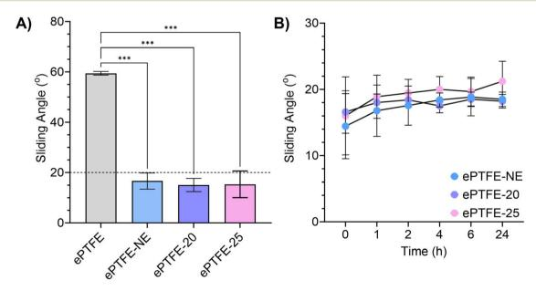
Fig. 3 (A) Initial sliding angle of the GSNO-NE-infused ePTFE samples and their controls. As observed, ePTFE alone has some level of slip; however, in introduction of the NE into the polymer matrix further decreased the sliding angle below 20 (n = 4, \*\*\*p < 0.001). (B) NE coating stability over 24 h. The slippery behavior of the NE-infused samples was maintained even after incubation at physiological conditions ( $n \ge 6$ , p > 0.05).
