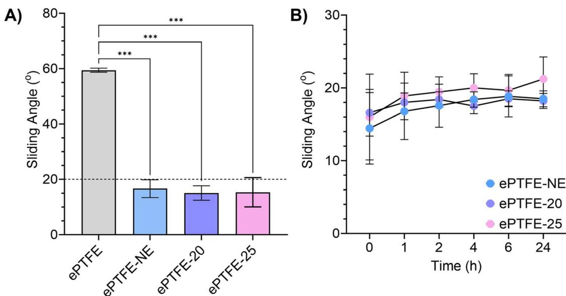
**Fig. 3** (A) Initial sliding angle of the GSNO-NE-infused ePTFE samples and their controls. As observed, ePTFE alone has some level of slip; however, in introduction of the NE into the polymer matrix further decreased the sliding angle below  $20^\circ$  ( $n = 4$ ,  $***p < 0.001$ ). (B) NE coating stability over 24 h. The slippery behavior of the NE-infused samples was maintained even after incubation at physiological conditions ( $n \geq 6$ ,  $p > 0.05$ ).
