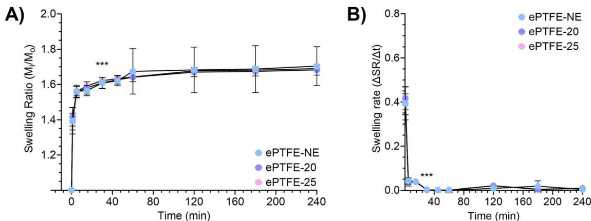
**Fig. 2** Swelling (A) ratio and (B) rate of ePTFE samples. Since the ePTFE, which is inherently hydrophobic, was especially porous, it was able to swell the hydrophobic NE within 30 min with no significant change in weight after that time ( $n = 6$ ,  $***p < 0.001$ ).
