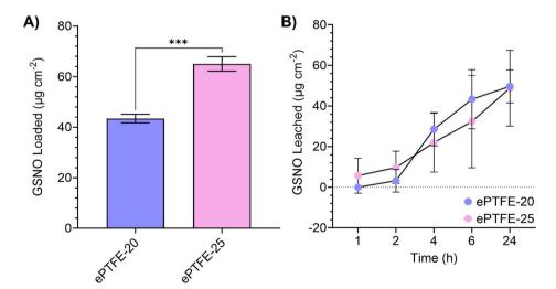
Fig. 4 (A) GSNO loading (n = 3, \*\*\*p < 0.001). (B) GSNO leaching (n = 3, p > 0.05). While the GSNO loaded into the ePTFE-25 sample was significantly higher than that of ePTFE-20, the leaching profiles are similar. Nearly all of the GSNO loaded into the NE and infused into the ePTFE was depleted after 24 h.
