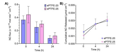
Fig. 5 (A) NO release over 24 h. (B) Cumulative NO released. Between both concentrations of GSNO loaded into the NE and infused into the ePTFE, there was no significant difference seen in the level of NO release. This is corroborated by the amount of GSNO diffused over 24 h ( $n \ge 5$ , p > 0.05).
