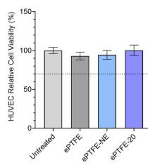
Fig. 6 (A) Relative cell viability of 3T3 cells and (B) HUVECs when exposed to GSNO-NE-infused ePTFE and its controls. The dashed line at 70% cell viability represents the ISO threshold for cell cytocompatibility. The addition of the NE, and subsequently GSNO, into the ePTFE did not cause significant decrease in cell viability as the NO released was not high enough to elicit cytotoxic effects (n = 4, p > 0.05).
