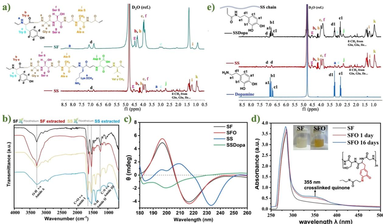
**Fig. 2** (a)  $^1\text{H}$  NMR spectra of extracted SF (green) and SS (red). (b) FTIR spectra of extracted SF and SS, compared with commercially available products. (c) CD spectra of extracted SF, SS and modified SFO, SSDopa at  $0.2 \mu\text{g ml}^{-1}$ . (d) UV-Vis spectra of SF and oxidized SFO after 1 day and 16 days. (e)  $^1\text{H}$ -NMR spectra of SSDopa, unsubstituted SS, and dopamine monomer.
