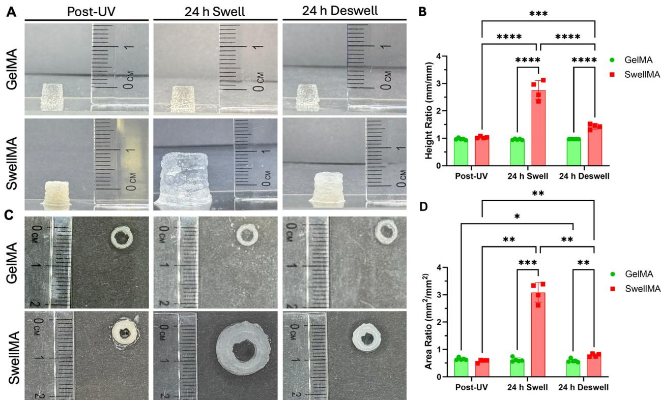
**Fig. 9** Cylinder print test of GelMA and SwellMA after UV crosslinking and after 24 h of swelling and shrinking. (A) Macroscopic profile images and (B) quantification of cylinder height ratio. (C) Macroscopic top view images and (D) quantification of the crosssectional area ratio. \*\*\*\*Denotes significance ( $p < 0.0001$ ), \*\*\* ( $p < 0.001$ ), \*\* ( $p < 0.01$ ), \* ( $p < 0.05$ ),  $n = 3$ , data shown as mean  $\pm$  SD.
