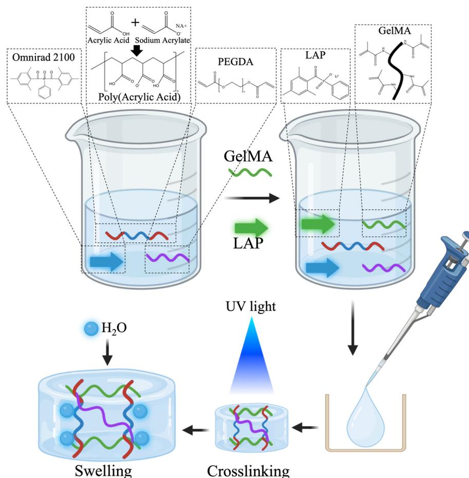
**Fig. 1** Schematic of SwellMA Synthesis. Poly(acrylic acid) was mixed with poly(ethylene glycol) diacrylate (PEGDA) and Omnirad 2100. Then GelMA and LAP were added to the solution and mixed until a homogeneous mixture was obtained. This solution was pipetted into geometrically defined molds and crosslinked using UV light. After photopolymerization, the resulting constructs were hydrated, causing water absorption and subsequent swelling.
