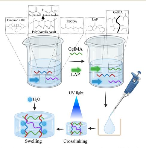
Fig. 1 Schematic of SwelMA Synthesis. Poly(acrylic acid) was mixed with poly(ethylene glycol) diacrylate (PEGDA) and Omnirad 2100. Then GelMA and LAP were added to the solution and mixed until a homogeneous mixture was obtained. This solution was pipetted into geometrically defined molds and crosslinked using UV light. After photopolymerization, the resulting constructs were hydrated, causing water absorption and subsequent swelling.
