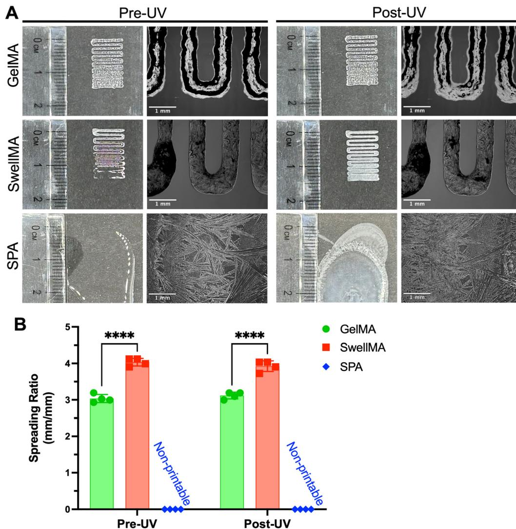
Fig. 7 Filament fusion and filament spreading test of GelMA, SwellMA, and SPA. (A) Macroscopic and microscopic images of filament before and after UV curing, scale bar = 1 mm. (B) Quantification of the filament spreading ratio. \*\*\*\*Denotes significance ( $p < 0.0001$ ),  $n = 4$ , data shown as mean  $\pm$  SD.
