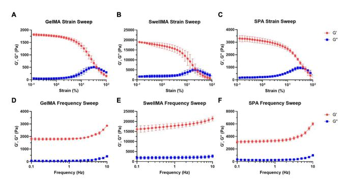
Fig. 5 Rheology characterization for GelMA, SwellMA, and SPA. (A–C) Strain sweep of GelMA, SwellMA, and SPA with 1 Hz frequency at 37 °C. (D–F) Frequency sweep of GelMA, SwellMA, and SPA with 1% strain at 37 °C. N = 3, data shown as mean  $\pm$  SD.
