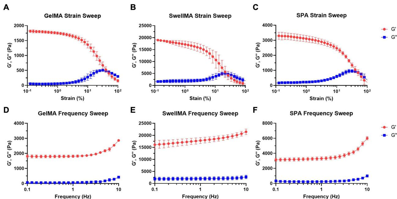
**Fig. 5** Rheology characterization for GelMA, SwellMA, and SPA. (A–C) Strain sweep of GelMA, SwellMA, and SPA with 1 Hz frequency at 37 °C. (D–F) Frequency sweep of GelMA, SwellMA, and SPA with 1% strain at 37 °C.  $N = 3$ , data shown as mean  $\pm$  SD.
