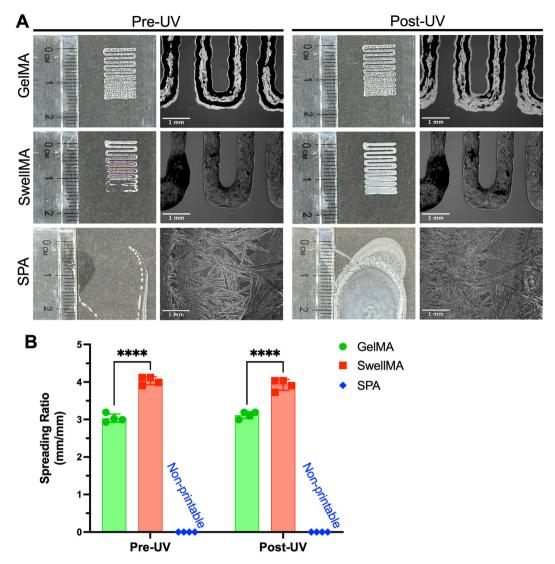
Fig. 7 Filament fusion and filament spreading test of GelMA, SwellMA, and SPA. (A) Macroscopic and microscopic images of filament before and after UV curing, scale bar = 1 mm. (B) Quantification of the filament spreading ratio. \*\*\*\*Denotes significance (p < 0.0001), n = 4, data shown as mean + SD.
