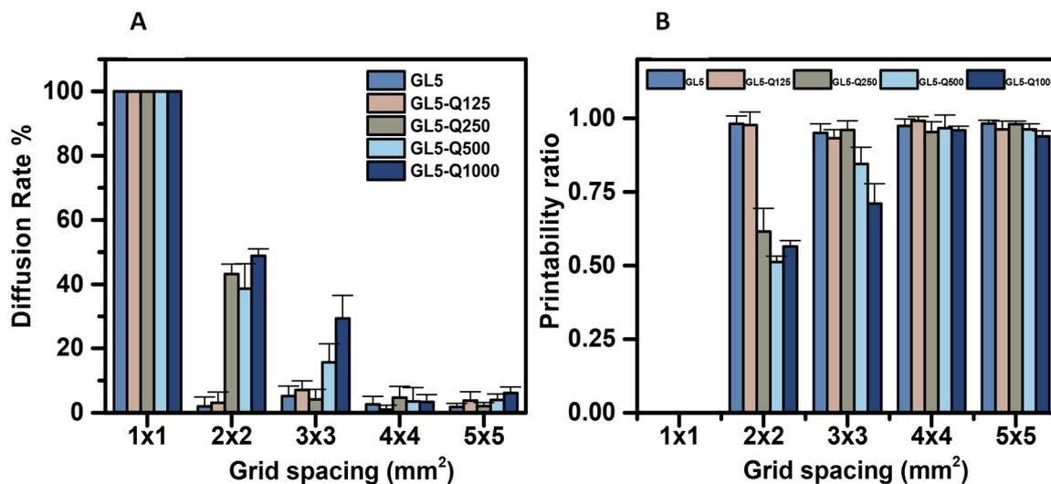
Fig. 3 Printability ratio (A) and diffusion rate percentage (B) of the GL5, GL5-Q125, GL5-Q250, GL5-Q500, GL5-1000 inks.
