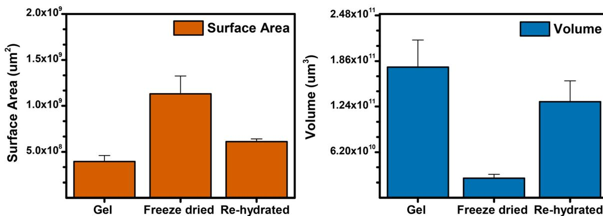
Fig. 5 Comparison of volume (left) and surface area (right) across different states—originally printed, freeze-dried, and re-hydrated. Measurements were obtained from X-ray CT analysis of whole-sample scans at a voxel resolution of 16.8 µm.
